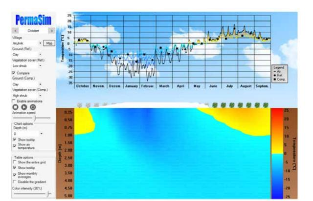
Figure 9. Example of a dsplay of PermaSim. Upper graph, annual air temperature curve (black) and two potential soil surface temperature curves depending on snow cover thickness selected by the student. Lower graph, annual evolution of the ground temperature profile. The simulation is animated on the computer screen.
