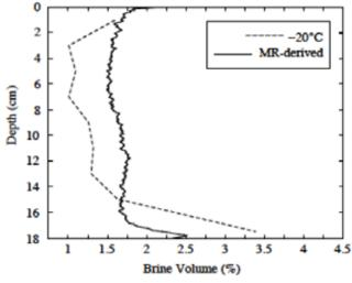
Figure 5. The brine volume (after Cox and Weeks, 1983) calculated using the observed bulk salinity data and the sample storage temperature of -20°C, to best approximate the brine volume of the sample as it was imaged by the MR scanner, and the liquid fraction at each of 290 rows (180.67 vertical mm) derived from the MR image data normalized by the highest voxel value.
