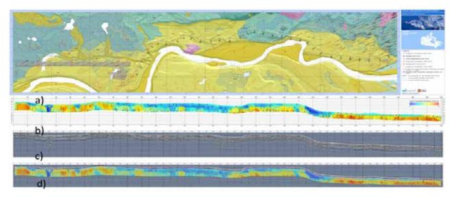
Figure 8. Permafrost characterization along the road to the airport, Tasiujaq, Nunavik. A) surficial geology map with locations of soundings, drillholes and survey pits. B) Capacity resistivity survey profile along the road. c) Ground penetrating radar profile. D) superposition of Resistivity and GPR profiles. (Figure produced by E. L'Hérault and team.)
