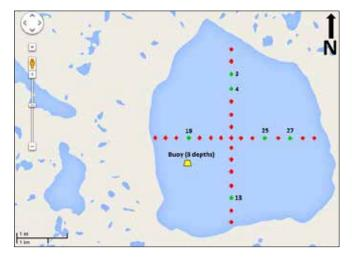
Figure 5. Schematic representation of the Noell Lake ice survey locations (red diamonds) used as water sample locations (green diamonds). Additional water samples were taken at sites proximate to the ALMS (yellow trapezoid).
