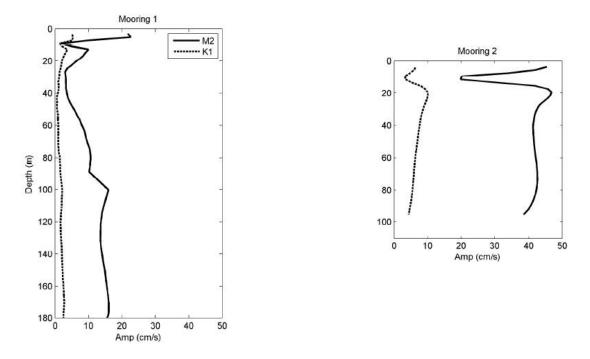
Figure 5. The vertical profiles of the amplitudes of the two primary tidal constituents, the semi-diurnal M2 component and the diurnal K1 component.
