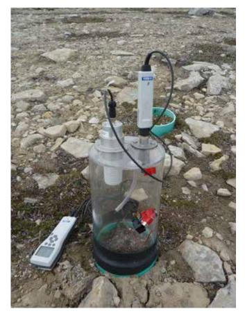
Figure 11. Static CO<sub>2</sub> measurement chamber measuring NEE (photo credit: Emma Buckley).
