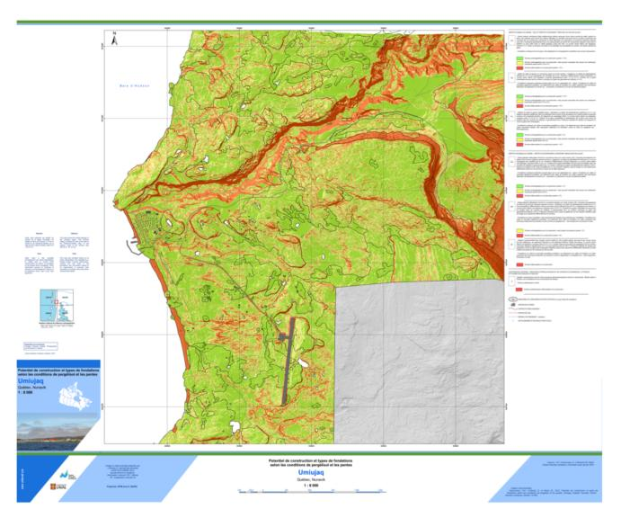
Figure 6. Map of potential for construction on permafrost of the community of Umiujaq, Nunavik.
