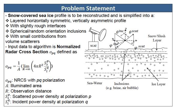
Figure 10. The simplified profile from which the forward and inverse model was developed.
