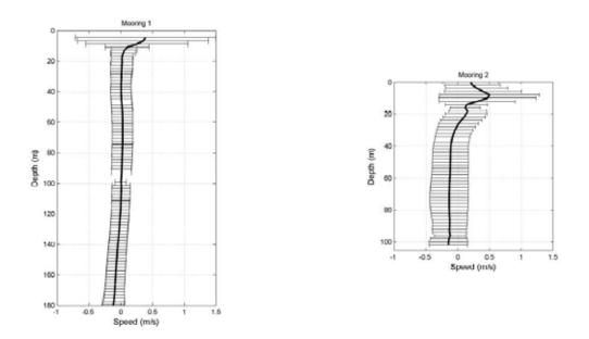
Figure 7. Averaged along-channel currents at the two mooring stations M1 and M2.
