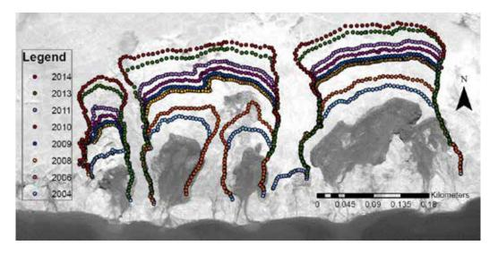
Figure 9. Locations of retrogressive headwalls between 2001 and 2014. Data collected in 2001 from satellite imagery and between 2004 and 2014 using differential GPS.
