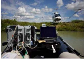
Figure 3. Sampling CO, flux from a permafrost thaw pond.
