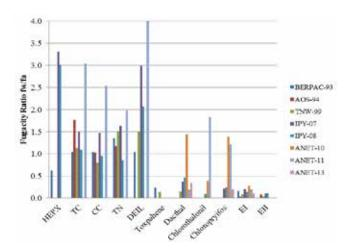
Figure 8. Fugacity ratio for OCPs and CUPs between 1993-2013, where 1.0 is equilibrium, <1.0 and >1.0 are deposition and volatilization, respectively. Fugacity ratios between 0.7-1.3 are not significantly different from 1.0.
