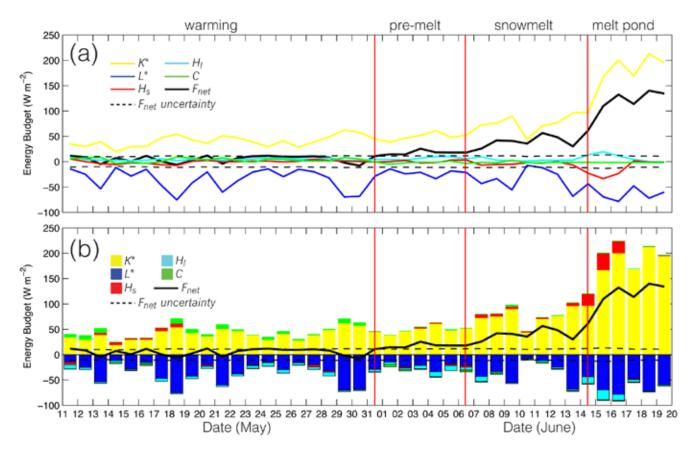
Figure 7. Two representations of the mean daily energy budget terms. In (b) the sign of the turbulent fluxes ( $H_s$  and  $H_p$ ) are reversed from the normal convention so that all sources of energy to the surface are displayed as upwards pointing bars (and vice versa). Red vertical lines are located at the first observations of positive surface temperature (June 1), snowmelt onset (June 6), and melt pond onset (June 14).
