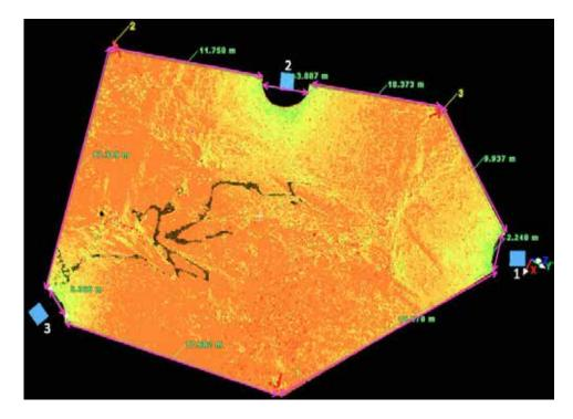
Figure 7. Point cloud model of the non-invasive sampling site in Dease Strait. Scanning platform locations are shown as blue rectangles and HDS target locations are shown as red tripods (yellow numbers point to the location). Measurement values around the sampling site are displayed in metres.
