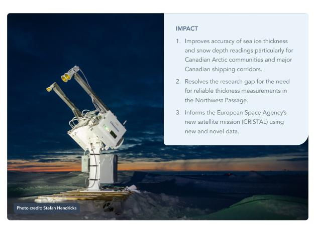
The KuKa radar is a surface-based dual frequency Ka/Ku-band radar that can be used to measure sea ice thickness.
