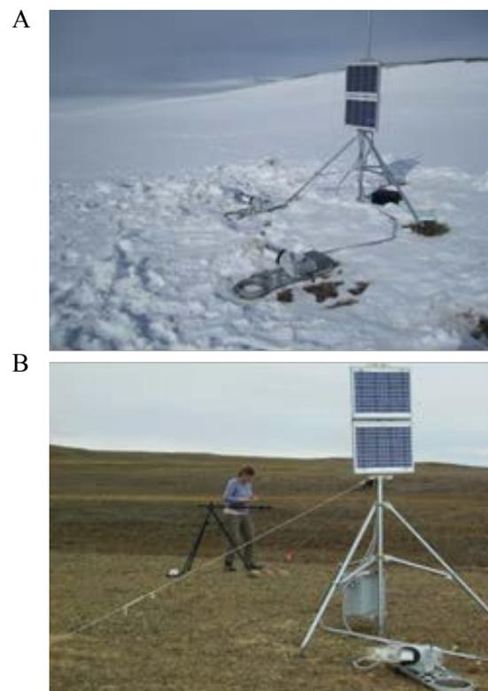
*Figure 4. A) Automated ACE systems measuring carbon fluxes from frozen ground B) ACE system on polar semi-desert community with NDVI measurements in the background.*
