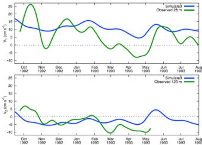
Figure 2a. Comparison between observed and simulated velocities at a northeastern Hudson Bay station.  $V_1$  ( $V_2$ ) is the velocity in the upper (lower) model layer. Data from the lower current-meter are not available after May 1993. Note the episodes of flow reversal in  $V_2$ .
