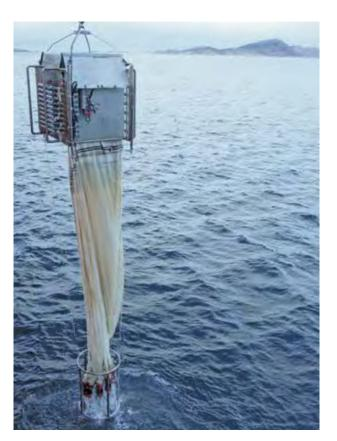
Figure 19. Vertical hydrobios multinet.
