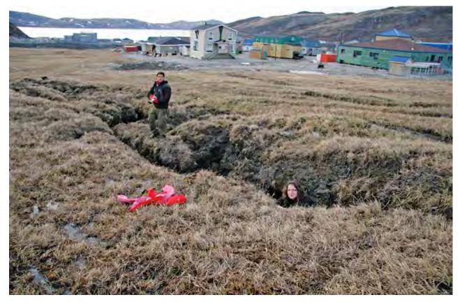
Figure 8. Thermal erosion process initiated by the passage of a heavy vehicle, Salluit.
