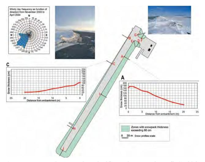
**Figure 5.** *Tasiujaq airstrip with two transects showing clear difference in the snow accumulation profiles (A and C) for both sides of the runway. Snow accumulation is directly affected by the dominant winds coming from the Southwest. Letters represent other transects of snow accumulation profiles.*
