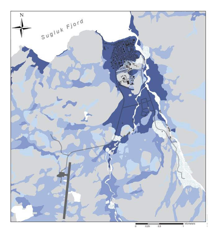
**Figure 10.** Map of permafrost conditions (ice content) in Salluit according to the spatial variability of surficial geology and geomorphologic features. Modified from Allard and L'Hérault 2010.
