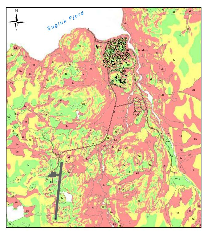
**Figure 11.** *Risk management map for potential construction development in Salluit. Derived from Allard and L'Hérault 2010.*
