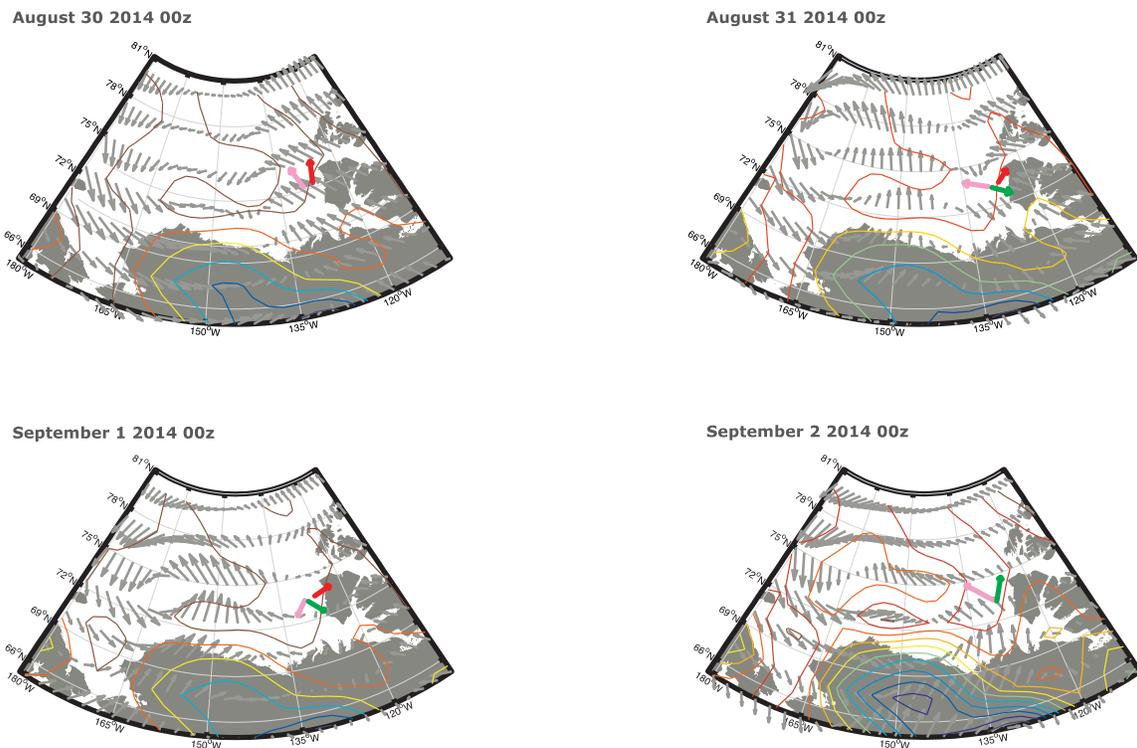
Figure 4. The wind fields and pressure fields from four days leading up to a strong wind event that destroyed one of the on ice towers. In situ wind vectors measured by the on ice towers are shown in pink, red and green, off the coast of Banks Island.
