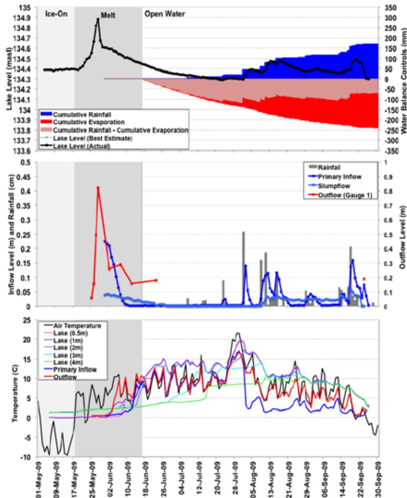
Figure 3b. (a) The Lake Level of Lake 5B from May 1st to September 30th, 2009, plotted with Cumulative Rainfall, Cumulative Evaporation, and Cumulative Rainfall – Cumulative Evaporation; (b) the water level of the Primary Inflow, Slumpflow, and Outflow, plotted with Rainfall; (c) Ambient Air Temperature, Lake Water Temperature (at 0.5 m, 1 m, 2 m, 3 m, and 4 m), and the temperature of the Primary Inflow and Outflow.
