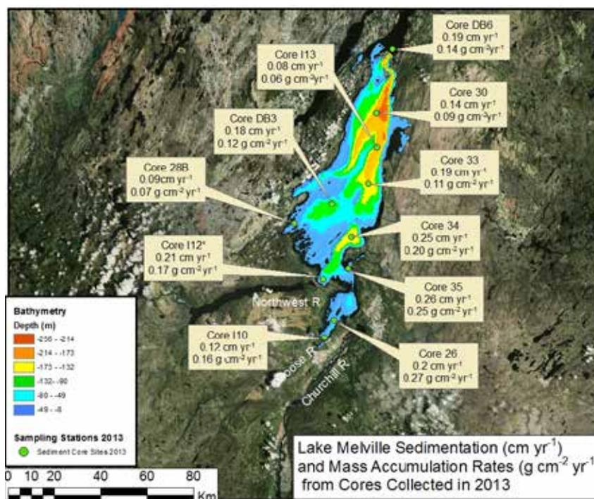
Figure 2. Map showing  $^{210}\text{Pb}$  estimated sedimentation ( $\text{cm yr}^{-1}$ ) and mass accumulation rates ( $\text{g cm}^{-2} \text{yr}^{-2}$ ) calculated from cores collected in June 2013.
