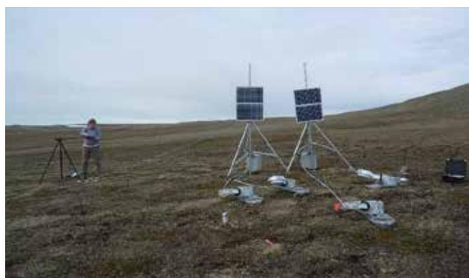
Figure 10. Static chamber system used to measure carbon exchange rates. Automated chamber systems measuring carbon exchange rates every 30 minutes.
