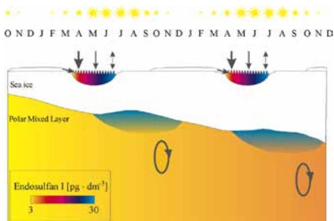
Figure 10. Hypothetical contaminant pump function schematic using endosulfan I as an example, colors denote endosulfan I concentrations in melt ponds and seawater.
