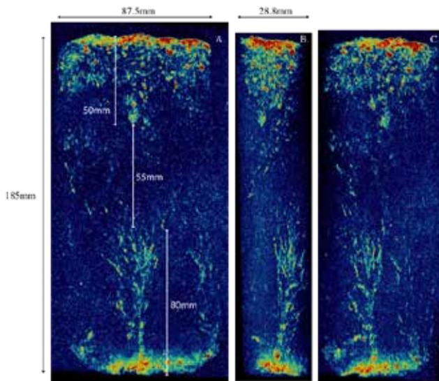
Figure 4. Magnetic resonance images in a 3-dimensional maximum intensity projection (MIP) made up of 72 images each with a thickness of 0.4 mm (Z) (28.8 mm total thickness) of a sea ice core (depth (Y) = 186 mm, diameter = 87.5 mm) viewed from the front (LEFT), side (MIDDLE) and rotated obliquely (RIGHT). These MR images can be used to compute liquid fraction profiles in sea ice (Figure 5).
