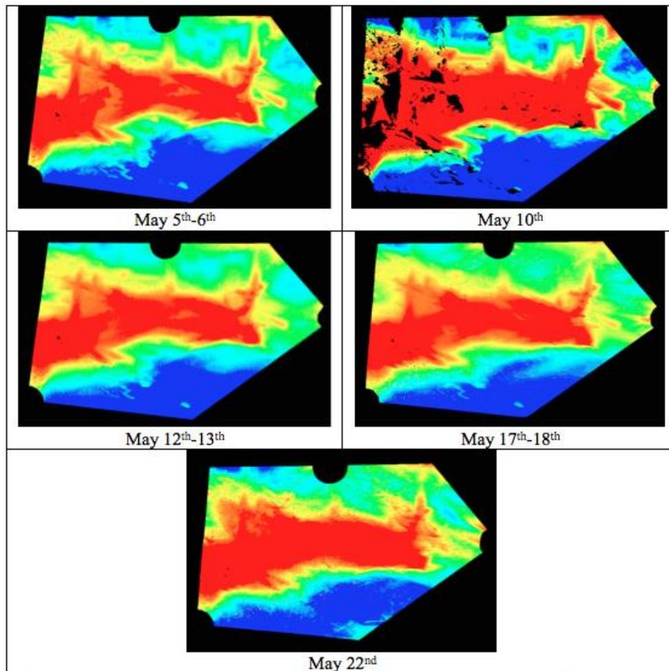
Figure 8. Point cloud models from Dease Strait mapped by elevation. Red represents areas of highest elevation and blue represents areas of lowest elevation.
