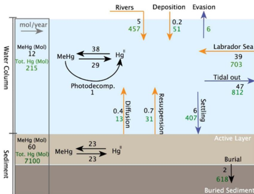
Figure 12. Empirically constrained annual mass budget for total Hg and MeHg in Lake Melville (from Schartup et al. submitted). Mass flow rates are shown as mol Hg a<sup>-1</sup> and reservoirs are given in moles. Orange arrows represent external sources of MeHg and total Hg to the water column and blue arrows represent losses.
