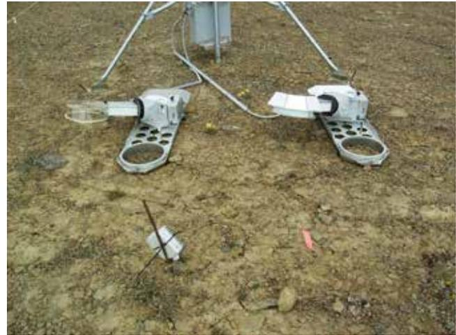
Figure 12. Automated CO<sub>2</sub> chambers with transparent and opaque covers (photo credit: Neal Scott).
