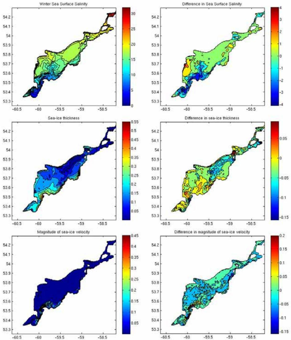
Figure 10. Model simulation of surface characteristics (left panels) of Lake Melville and their differences (right panels) in the two experiments with different river discharge.
