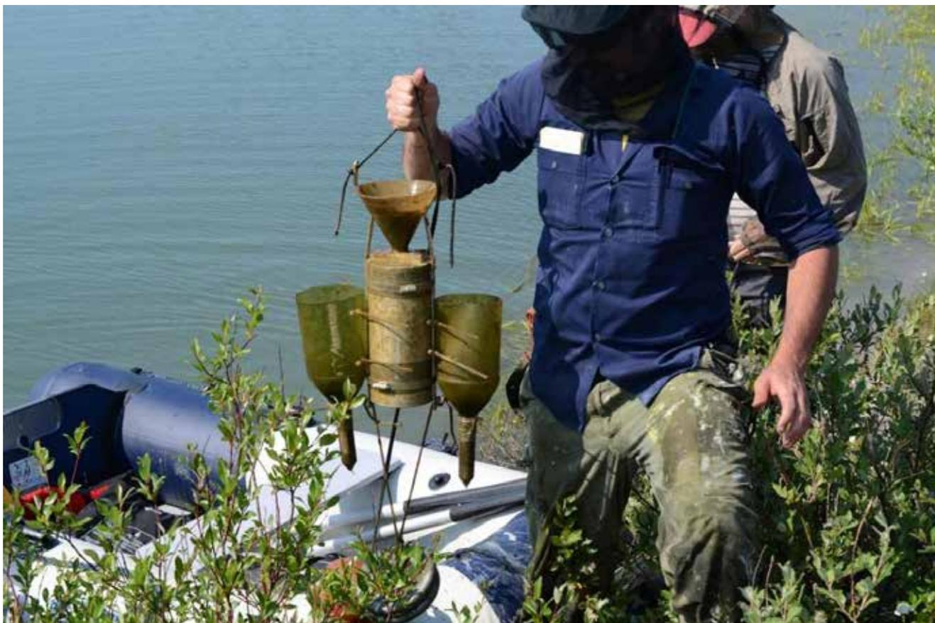
*Figure 10. Sediment trapping system installed at the 'BGR A' site (ADAPT Super Region), near Umiujaq (Eastern Hudson Bay). An optical trap (center), equipped with a collecting funnel, records sedimentological events throughout the year, while two side 'home-made' traps sample settling material during the same period. Photo: A. Matveev.*
