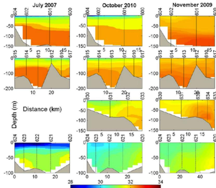
Figure 8. Salinity contours for four Labrador fjords. Each row of panels is from the same fjord, starting from the northernmost fjord (Nachvak) at the top and moving south to Saglek, Okak and then Anaktalak at the bottom. The columns are sorted by season, starting with July on the left (2007) and moving to October (2010) and November (2009). Vertical lines indicate the location of the sampling stations (numbers).
