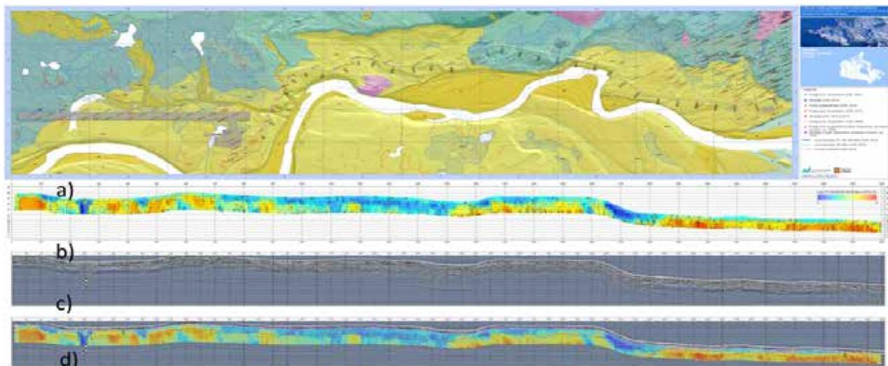
Figure 8. Permafrost characterization along the road to the airport, Tasiujaq, Nunavik. A) surficial geology map with locations of soundings, drillholes and survey pits. B) Capacity resistivity survey profile along the road. c) Ground penetrating radar profile. D) superposition of Resistivity and GPR profiles. (Figure produced by E. L'Hérault and team.)
