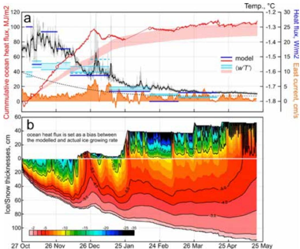
Figure 3. (a) The cumulative oceanic heat influx evaluated as a bias between the modeled and measured sea-ice thicknesses at m04. The grey and black curves specify the surface water temperature and its 24-h running mean; dashed black line is freezing point at the surface. The eastward currents from 6-m depth (cm/s) are shown in orange. (b) The temporal evolution of modeled ice/snow temperature distribution.
