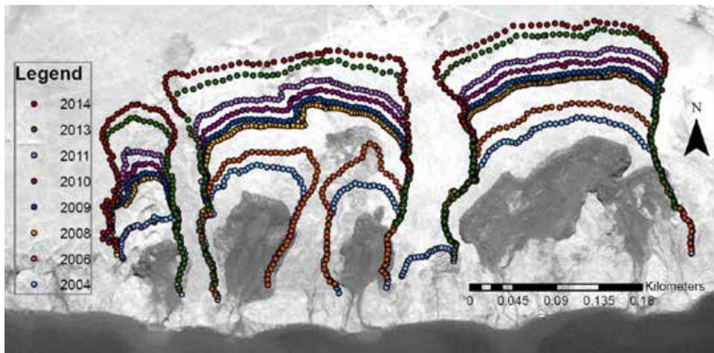
Figure 9. Locations of retrogressive headwalls between 2001 and 2014. Data collected in 2001 from satellite imagery and between 2004 and 2014 using differential GPS.
