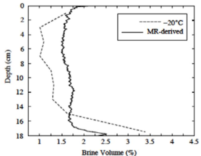
Figure 5. The brine volume (after Cox and Weeks, 1983) calculated using the observed bulk salinity data and the sample storage temperature of  $-20^{\circ}\text{C}$ , to best approximate the brine volume of the sample as it was imaged by the MR scanner, and the liquid fraction at each of 290 rows (180.67 vertical mm) derived from the MR image data normalized by the highest voxel value.
