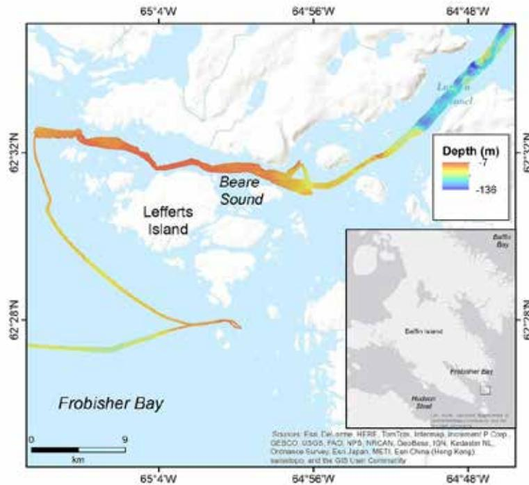
Figure 15. Multibeam coverage of transit corridor and anchorage locations within Bear Sound, through Anderson Channel. Inset is a map of southern Baffin Island, with the location of Anderson Channel outlined at the southeast extent of Frobisher Bay.
