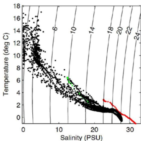
Figure 4. T-S diagrams of CTD data collected along the center of the Lake and Narrows from June to July 2013. The green dots are from M1, inside The Narrows; the red dots are from M2 outside The Narrows.
