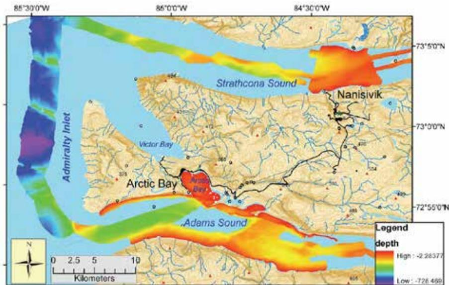
Figure 11. Map showing multibeam bathymetric coverage for Adams Sound, Strathcona Sound, and Arctic Bay. The Arctic Bay habitat mapping project focuses exclusively on Arctic Bay itself and the adjacent shallow waters of Adams Sound. Maximum depths within the bay are 100 m.
