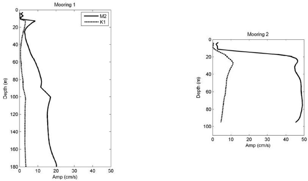
Figure 6. The amplitudes of the two key tidal constituents when ice is present in the Lake.
