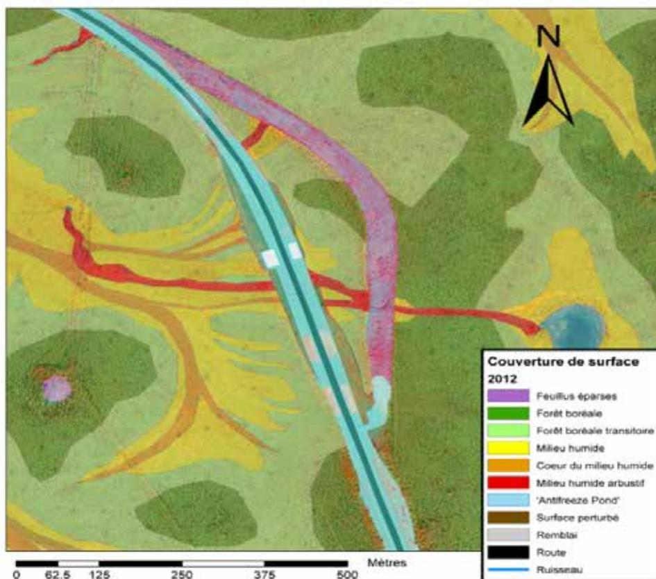
Figure 5. Eco-geomorphological map of discontinuous permafrost terrains (Beaver Creek, YT) showing the interaction between terrain units and the road infrastructure (M. Sliger).
