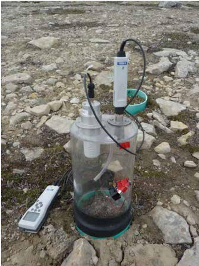
Figure 11. Static CO<sub>2</sub> measurement chamber measuring NEE (photo credit: Emma Buckley).
