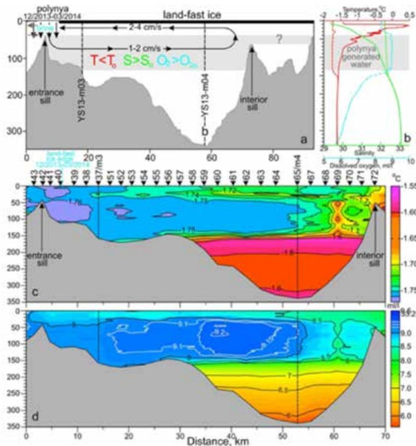
Figure 2. (a) Schematic depiction of polynya impact on circulation in Young Sound, (b) vertical distribution of temperature (red, °C), salinity (green) and DO (blue, ml/l) in 10/26/2013 (solid lines) and 5/5/2014 (dashed lines) at mooring m04, (c-d) along-fjord transect of temperature and DO. From Dmitrenko et al., 2015. © 2014 Elsevier Ltd. All rights reserved.
