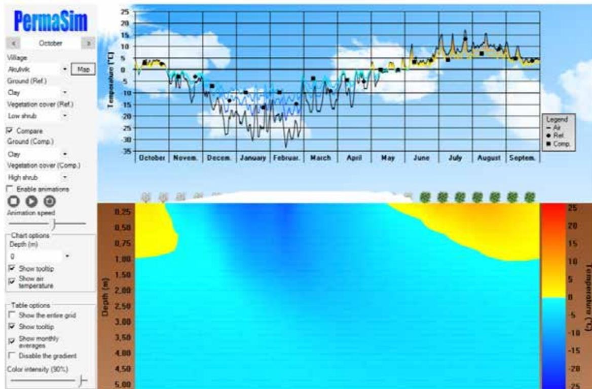
Figure 9. Example of a display of PermaSim. Upper graph, annual air temperature curve (black) and two potential soil surface temperature curves depending on snow cover thickness selected by the student. Lower graph, annual evolution of the ground temperature profile. The simulation is animated on the computer screen.
