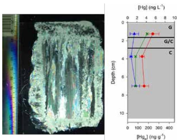
Figure 1. Distribution of mercury in experimental sea ice at SERF, showing the texture of sea ice (left) and the dominance of particulate mercury (right) (from Beattie et al., manuscript in preparation).
