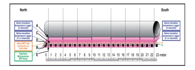
Figure 9. Scheme of the Abem Terrameter LS system used in the electrical resistivity tomography (ERT) surveys.
