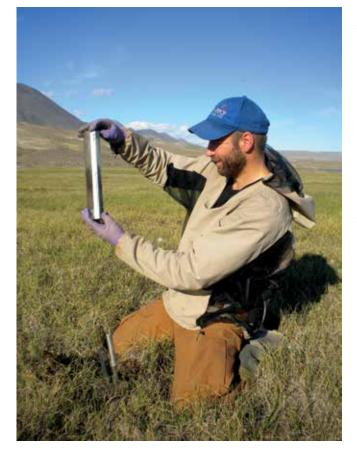
Figure 4. Igor Lehnherr holding a peat core from the wetland in the Skeleton Lake subcatchment that was used for mercury methylation incubation experiments (Credit: V. Wisniewski).
