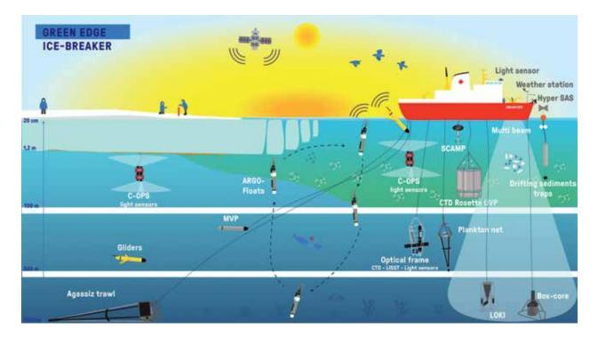
Figure 4. Visual summary of the equipment used during the GreenEdge oceanographic cruise (credit: Julie Sansoulet).
