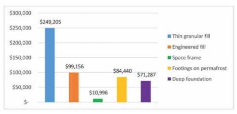
*Figure 3. Expected (discounted) lifetime costs of climate change for housing built on different types of foundation (average cost per house) (from Bell et al. 2016, submitted).* © 2016 Bell, Dion, Kors-Olthof, Perrin, Riedlsperger, Trimble.
