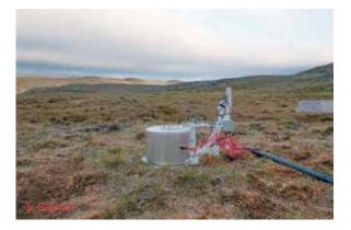
Figure 12. Automated chambers to detect and measure permafrost soil respiration.
