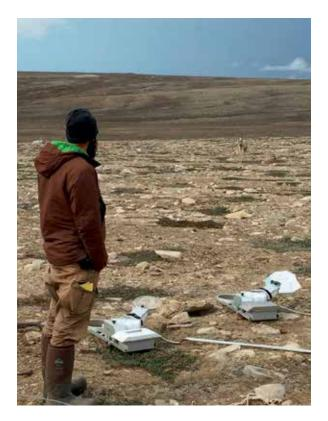
*Figure 1. Automated chamber systems measuring net carbon dioxide fluxes from polar semi-desert communities at the CBAWO. Even the wildlife like to observe research. Photo by Robert Mactavish.*
