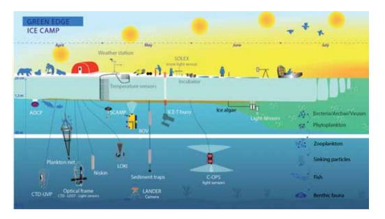
Figure 2. Visual summary of the instruments used during GreenEdge ice camp operations in 2016 (credit: Julie Sansoulet).
