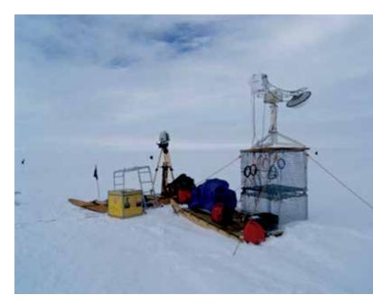
*Figure 1. On-site measurements of the scatterometer and lidar from the snow-covered sea ice at Cambridge Bay, Nunavut on May, 2014.*
