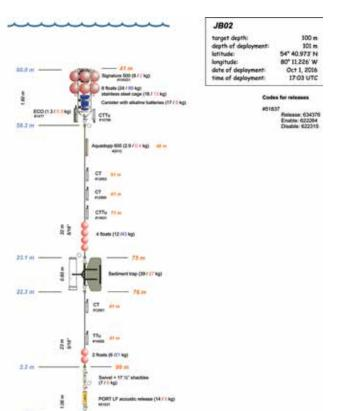
Figure 2. Mooring diagram for the mooring installed at the mouth of James Bay October 1, 2016, in partnership with the NSERC BaySys CRD project (D. Barber, Lead).
