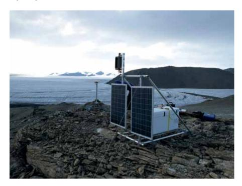
Figure 2. GPS unit installed on a rock outcrop along the edge of the Gilman Glacier (Credit: A. Dubnick).
