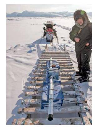
*Figure 2. SmartICE local research coordinator Andrew Arreak using SmartQAMUTIK to measure sea-ice thickness on Eclipse Sound near Pond Inlet, Nunavut (photo: SmartICE 2016).*
