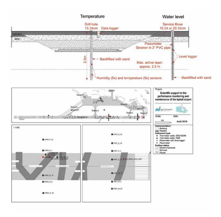
Figure 10. Thermistor cables installed in repaired cracks across the runway in Iqaluit.
