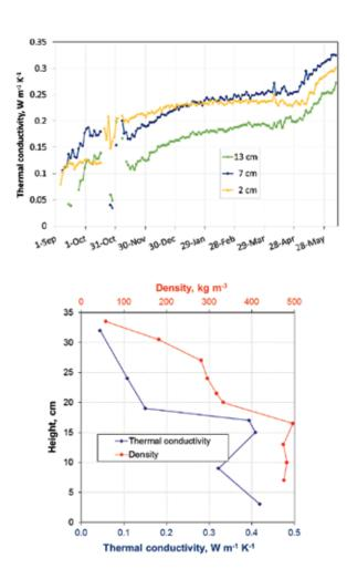
Figure 5. Measurement of snow physical properties at Ward Hunt Island. Top: continuous thermal conductivity measurements at three heights above ground, showing high values even at the very base of the snowpack. Bottom: vertical profile of snow density and thermal conductivity on thin rocky soil at a nearby spot (Source: Florent Domine, CEN/ ArcticNet).
