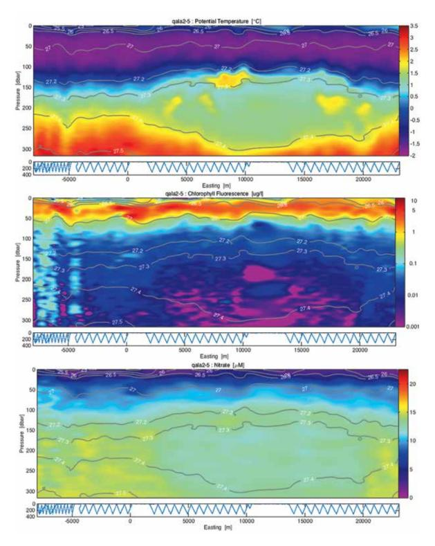
*Figure 41. Temperature, chlorophyll fluorescence and nitrate concentration along a glider transect during the GreenEdge oceanographic cruise.*
