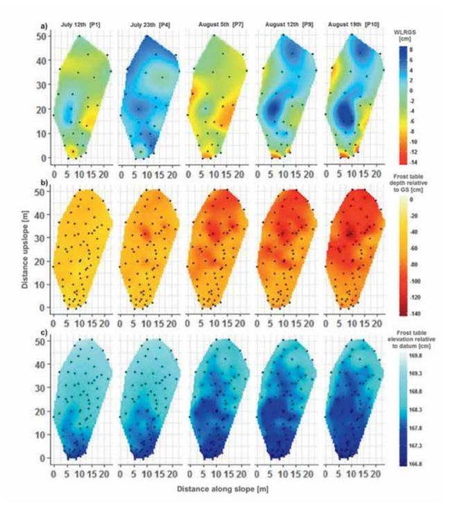
*Figure 16.* Nearest neighbour's interpolation showing the evolution of hillslope: *a*) piezometer water level relative to ground surface (WLRGS); *b*) frost table depth relative to ground surface (GS); and (*c*) frost table topography relative to local datum for a selection of 5 of the 10 sequential monitoring periods (i.e., P1, P4, P7, P9, P10). Black dots show measurements locations.
