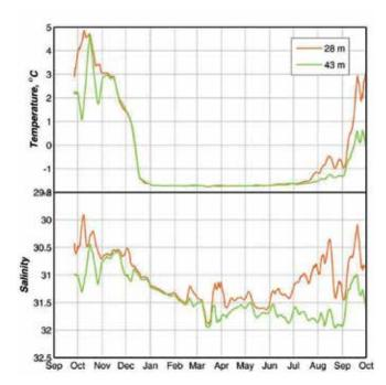
*Figure 5. The one-year evolution of vertical thermohaline structure at NE03 mooring.*
