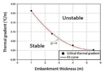
*Figure 8. Critical thermal gradient (yearly average) as a function of embankment thickness, to estimate heat balance at the soil/embankment interface.*
