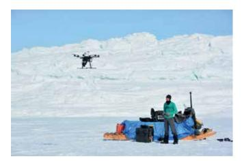
*Figure 8. Adam Garbo operating the uninhabited aerial vehicle (UAV) equipped with a camera and high-precision GPS on the sea ice in Frobisher Bay. Photo credit: M. St.Amant.*
