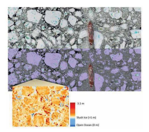
*Figure 2. UAV original imagery (top), polygon representation of ice floes and melt ponds (middle) and DEM for a subset of the survey area (bottom).*
