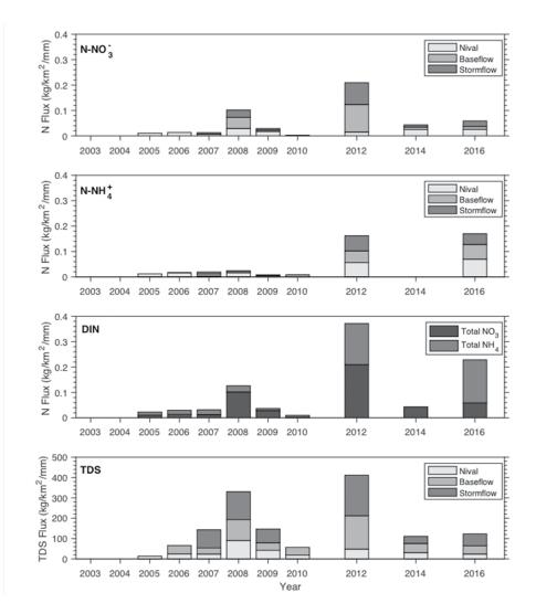
Figure 7. West River seasonal fluxes of  $N-NO_3^-$ ,  $N-NH_4^+$ , and TDS divided into nival, baseflow, and stormflow periods. Total  $N-NO_3^-$  and  $N-NH_4^+$  were summed to calculate DIN total. Samples were not collected in 2011, 2013, and 2015. Note the increase of  $N-NO_3^-$  and TDS fluxes in 2008, and the peak of  $N-NO_3^-$ ,  $N-NH_4^+$ , and TDS in 2012.
