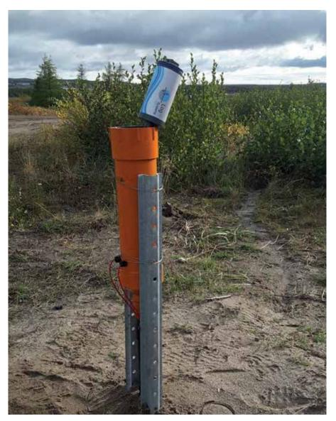
Figure 10. The UlogC16-32 from LogR Systems being set into a thermistor cable casing.
