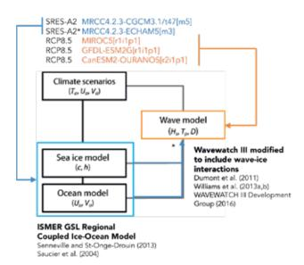
*Figure 1. Schematic showing the atmospheric, coupled iceocean and wave model simulations realized during the project and their dependencies.*
