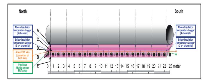
Figure 7. Design of the km 381 culvert monitoring setup.
