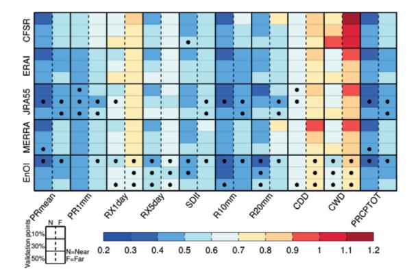
Figure 10. Normalized Root Mean Square Differences (NRMSD) over all validation sites for the period (1980-2009) (equation 1) for each indicator (x-axis). Near (N) and Far (F) configurations with 10, 30 and 50% of validation sites after applying OI to each reanalysis (top four rows) and after applying EnOI (bottom row). Black dots identify the datasets with the best performance (smallest NRMSD values) for a given subnetwork (N or F with 10, 30, or 50% validation points) and indicator.
