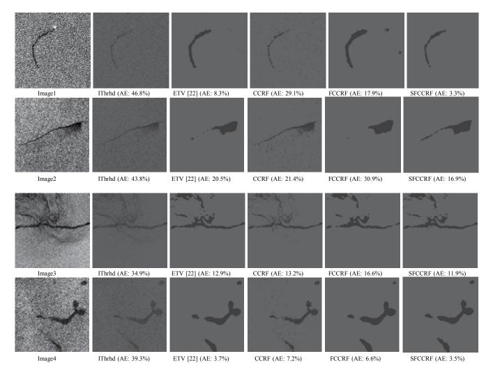
Figure 4. Detection of oil spill candidates by five different methods on four images. Comparing with the other methods, the proposed SFCCRF method is less affected by the background and target heterogeneities, and in the meantime can more accurately identify the boundaries and the linear targets.
