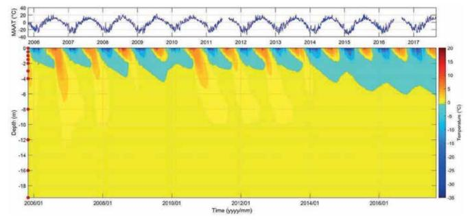
*Figure 5. Time-graph of ground temperature at the Biscarat site (0-20 m deep). Starting in 2014, permafrost has begun to form in the emerging coastal sediments, now reaching 6 m in thickness.*
