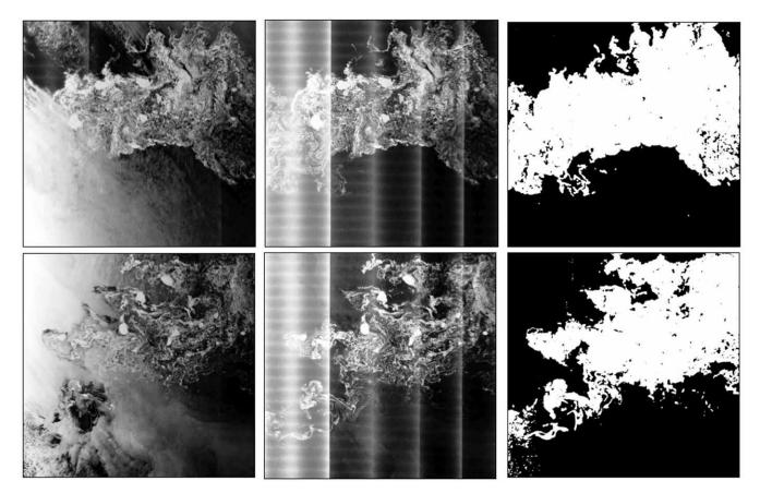
Figure 3. Two examples of successful application of a trained CNN applied to two ENVISAT SAR scenes. First column is the HHpol, second column is the HV-pol, and the third column is the output of the CNN successfully identifying ice and water regardless of the high noise content of the HV-pol. This is a demonstration of the success of using novel machine learning methods to the problem of binary ice/water segmentation and classification.
