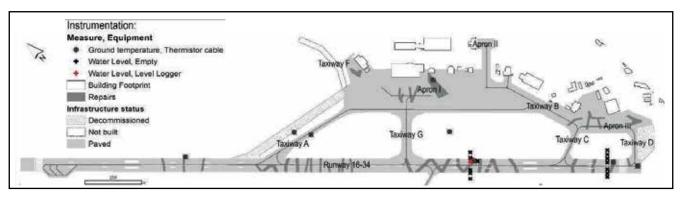
*Figure 9.* Map of changes and repairs done at Iqaluit airport to upgrade the facility and adapt it to climate warming. The map shows also the location of the monitoring instrumentation listed in the table.
