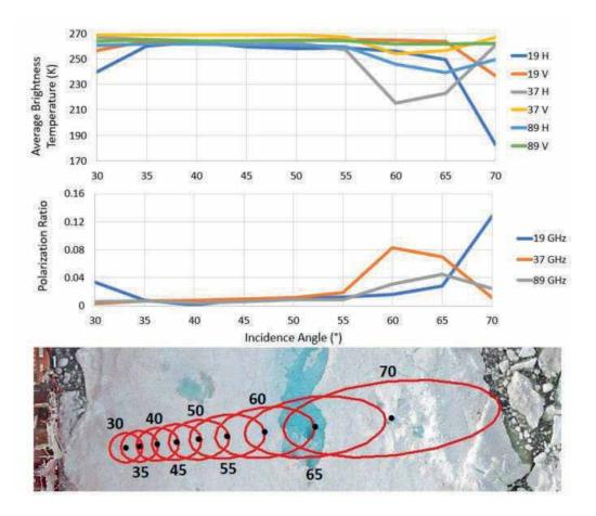
*Figure 1. Brightness temperatures (top) and polarization ratios (middle) plotted for each incidence angle, along with the FOV footprint for each angle shown across the scanned floe.*
