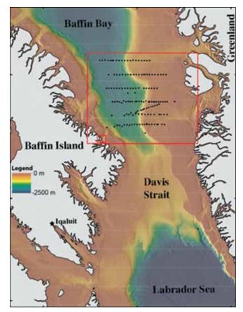
Figure 3. Map illustrating the sampling grid used during the GreenEdge oceanographic cruise on the CCGS Amundsen (red square). Bathymetric data is from the high resolution multibeam echosounder installed aboard the CCGS Amundsen (Gabriel Joyal and Patrick Lajeunesse) and the International Bathymetric Chart of the Arctic Ocean (IBCAO).
